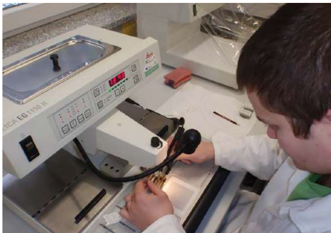
Fixation of decalcified tissue into wax using the embedding line LEICA EG 1150 H.
