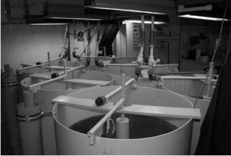
Fig. 23. Recirculating aquaculture system used for intensive rearing of pike ( Esox lucius L.) to the advanced fry (photo: T. Policar).
